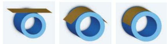
FIGURE 3. Slumping thin glass over Wolter Type-I molding die [4].
