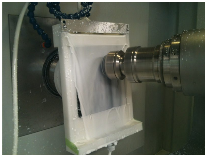
Figure 1: EUV Photomask on 7-Axis CNC Bonnet Polisher
