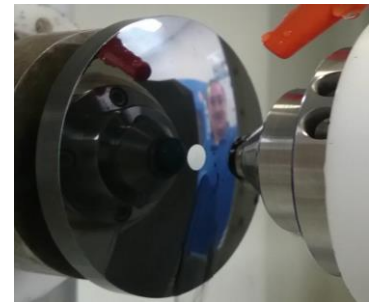
Fig. 3. Aspheric optic before and after SAG grinding
