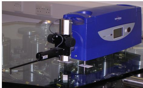
Fig. 4 Form Talysurf Intra stylus profilometer to measure edge profiles
