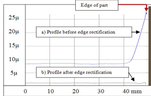
Figure 3 Profile before and after edge rectification
