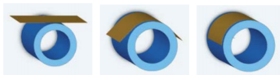
Figure 4. Principle of replication by slumping a thin glass sheet (~0.2 mm thick) over a molding die [7].
