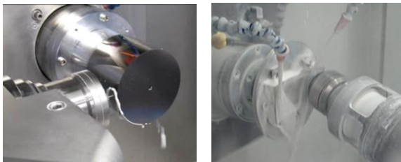
Fig.1. Fluid Jet and Bonnet Polishing on common 7-axis CNC machine
