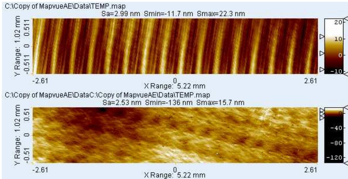
Fig. 2. Profilometer measurements of a raster polished region (top) and random polished region (bottom)
