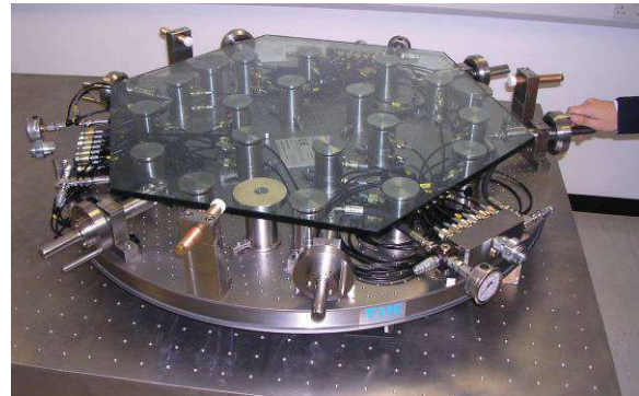
FIGURE 4. Original prototype hybrid lockable hydrostatic support system.
