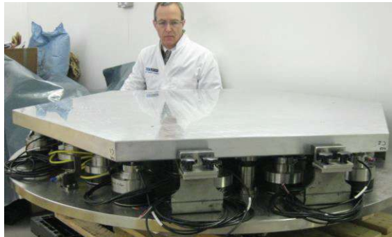
FIGURE 5. Dummy full-size segment integrated with polishing/metrology support system.
