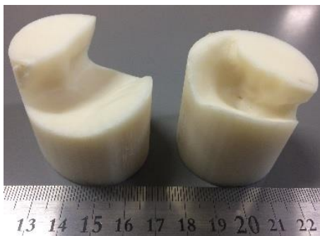
Figure 3: Holders with reverse shape of liver model
