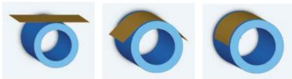
Fig. 1. Slumping process for 0.2mm thick LCD glass over fused silica mandrel.
