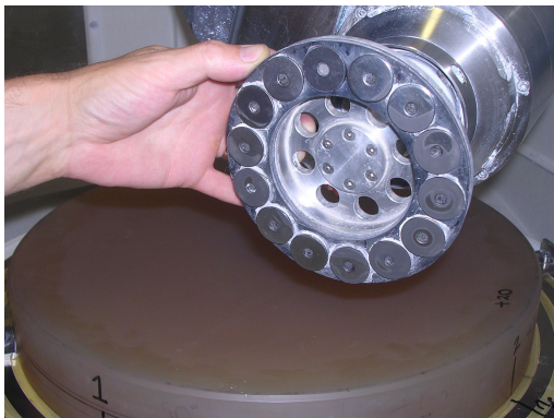
Figure 8 Ring tool on the 600mm machine, with the 500mm diameter part
