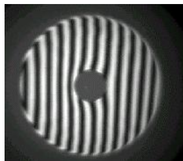
Figure 9 Interferogram of central plug after polishing spherical
