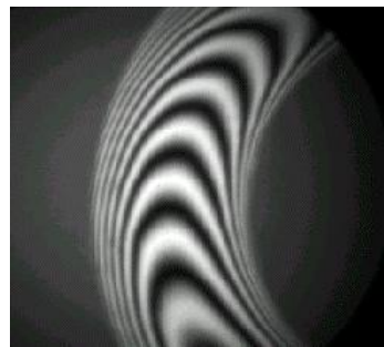
Figure 7 Interferogram of one side of 300mm part after aspherising
